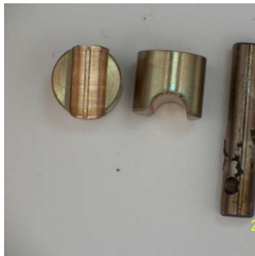
Failed pins following testing - note: Vee blocks should be Vee' d, not rounded -
